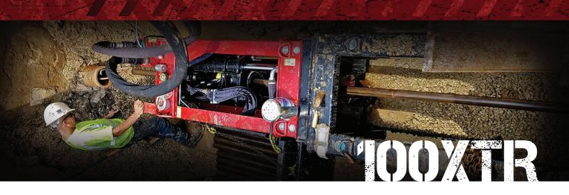
**AUTOMATED ROD SPINNER.** The innovative rod spinner system can thread and unthread rod during push or pull operations as rod is fed in from behind and a locking jaw system provides constant tension on the rod string which eliminates rod rebound. The result: no time wasted on stopping the burst for each rod.
