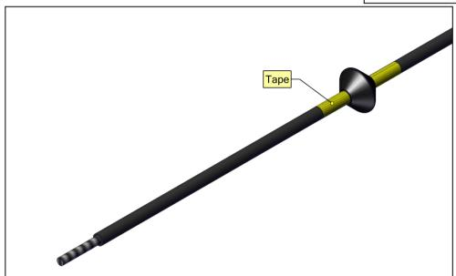
**Step 3.** Add Second Centraliser, Spacer Collet and Hub. Push Centraliser against the outer casing.
