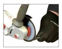
Always inspect the flexible shaft before each use. If there are potential weak points or the shaft is damaged, cut off the damaged length using an angle-grinder. This should be done outside in a clear area as there will be sparks generated by the process.
