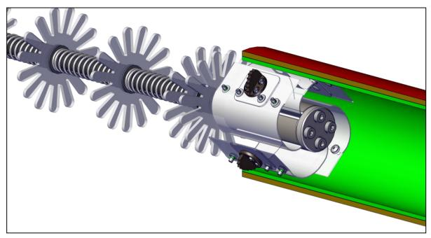
**Step 2.** Use a CCTV camera to measure the cutting spot. Push the Pipe Cutter into correct spot. Use a low rotation speed when positioning the Pipe Cutter in the correct spot. When the tool is in correct place, change the rotation speed to maximum. Use the CCTV camera monitor the cutting process. **Do not let the tool move while cutting. Never work blind!**
