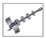
Do not pull back the Pipe Cutter from the main unless the cutter is turning at low speed. If the cutter is not running at a low rpm while pulling it back, the Pipe Cutter panels will spring open into the main. It will then be difficult to pull it back into the lateral. Running the Pipe Cutter at low rpm will help to collapse the panels back around the hub for easy removal.
