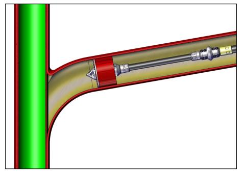
Step 2. Carefully drill the hole. Continue to push through so that you remove as much the liner away from the connection as possible. **Beware that you do not damage the already lined pipe during the process.** Use Smart Cutter<sup>™</sup> grinding panels to grind the hole edges before removing the tool from the pipe.
