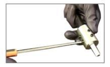
Feed the shaft through the socket to the end and **securely fasten**. The outer casing should reach all the way to the base of the shaft socket to protect the shaft.
