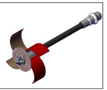
is also very effective for removing tree roots from the pipes. The front grinding discs are available in metal and plastic forms. Metal panel is more aggressive compared to the plastic panel. The diameter of the grinding discs is dependent on whether it is being used in a lined or unlined pipes (DN100 (4") and DN150 (6") pipe sizes). The smaller size plate should only be used in lined pipes.
