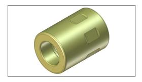
Always use a Sleeve Bearing when working with the Super Midi Miller or Super Midi Miller +C. It prolongs the lifetime of the flexible shaft and prevents the outer casing from melting in the tool end. Sleeve bearings can be reused when outer casing has been shortened.
