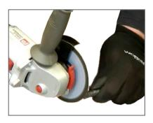
Before use always inspect the flexible shaft. If there are potential weak points or the shaft is damaged, cut off the damaged length using an angle-grinder. This should be done outside, in a clear area, as the process will generate sparks.
