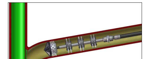
Step 2. Carefully drill the hole. Continue to push through so that you remove as much the liner away from the connection as possible. **Beware that you do not damage the already lined pipe during the process.** When you are satisfied with the opening, use Smart Cutter to grind the edges in the end.
