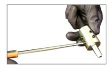
Feed the shaft through the socket to the end and **securely fasten**. To protect the shaft the outer casing should reach all the way to the base of the shaft socket.
