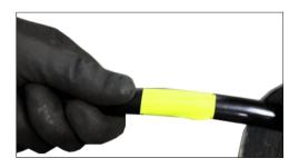
For your safety attach a visual marker (tape) to the outer casing of the flexible shaft. Place it around half a meter from the end point of the shaft. The marker will indicate the tool's location and prevent possible injuries, from the rotating parts, when the tool is removed from the pipe.
