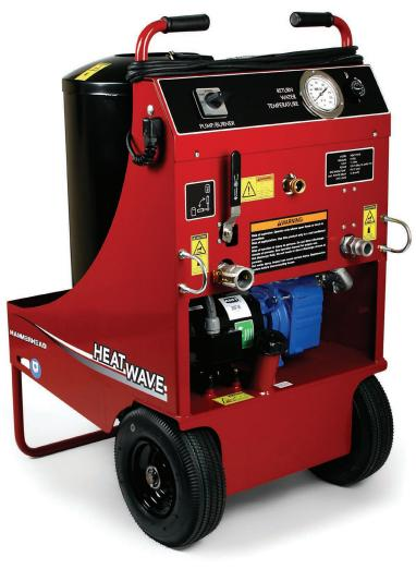
INTEGRATED DESIGN. The HeatWave incorporates the boiler and the pump in a single unit, simplifying setup, reducing the number of hoses to connect and maintaining a tidy footprint. Controls are centrally located for greater ease-of-use, and an onboard return temperature sensor makes monitoring effortless, so you can simply and precisely match the curing schedule. The boiler runs on diesel fuel and its pump runs on conventional 120 V power sources.
