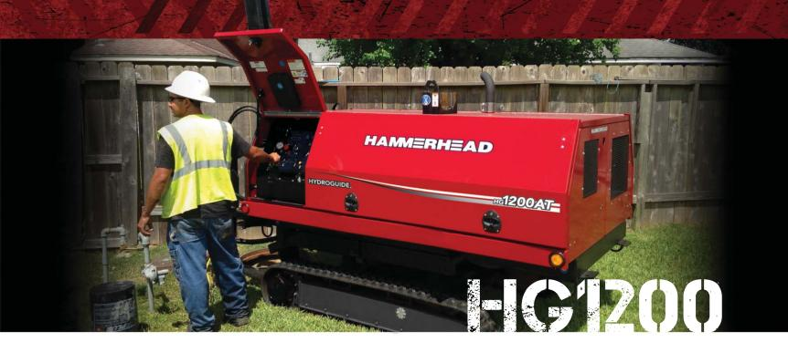
**AUTO BOOM.** While other winches require manual assembly of heavy, bulky downhole components, the HG1200 makes set up easy, safe and efficient with its patented, self-deploying hydraulic downrigger. With the touch of a button, operators can deploy the boom and fine-tune the depth without having to jack up the machine. Setup and teardown take just minutes which saves valuable time on a jobsite.
