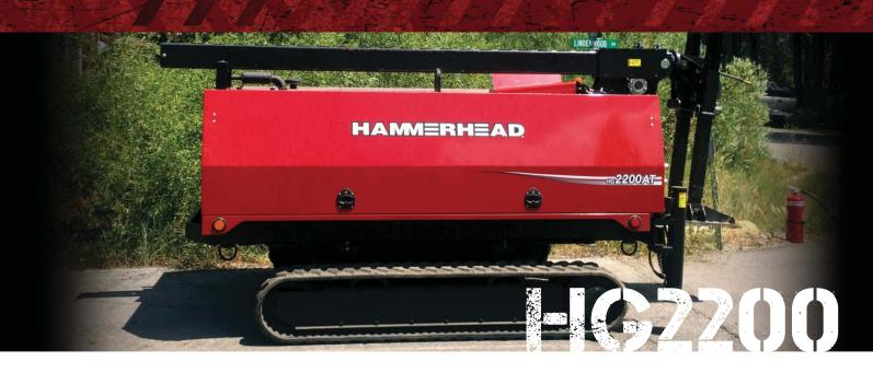
**PRODUCTIVITY IS TOP PRIORITY.** When it comes to time-saving, easy to use features, no other winch comes close. That's why the HG2200 comes standard with multi-position hydraulic levelling jacks, full radio remote control, auxiliary hydraulic power, remote electric start and remote operation for the deployable mast.
