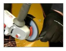
Always inspect the flexible shaft before each use. If there are potential weak points or the shaft is damaged, cut off the damaged length using an angle-grinder. This should be done outside in a clear area as the process will generate sparks.
