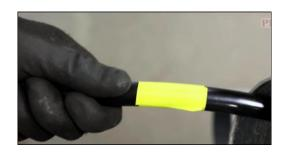
For your own safety attach a visual marker (tape) to the outer casing of the flexible shaft. Place it around half a meter from the end point of the shaft. The mark will indicate the tool's location and prevent possible injuries when a tool is removed from the drain, including injury by rotating parts.
