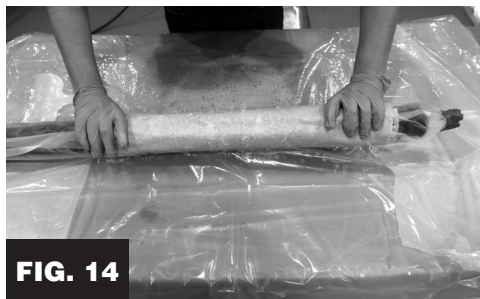
FIG. 11 Wet out both sides of matting
