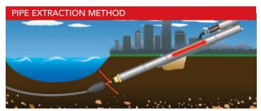
Recover your product pipe using the extraction method. The impact force of the rammer is combined with static pullback to extract product pipe so you can save expensive pipe and bore again.
