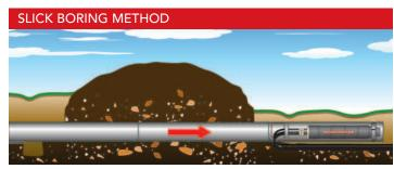
After installing a bore pipe using the conventional pipe ramming method, a new product pipe is pulled in using the pipe extraction method. This method is commonly used when specifications call for little or no impact on the carrier pipe weldments
