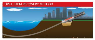
Recover your expensive, stuck drill stems! Attach the rammer to the drill stem with a fabricated adapter. The impact force of the rammer combined with static pullback is used to extract stuck drill stems.
