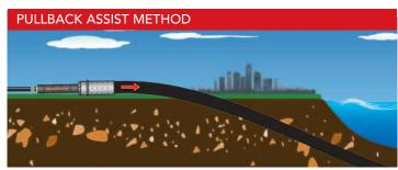
Free up hydro-locked or immovable pipe. The rammer is attached to product pipe during pullback and impact force assists HDD pullback to complete long and difficult projects.
