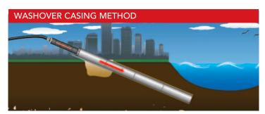
Start your job off right in tough conditions. Casings are rammed through difficult soil conditions to more desirable drill starting points. The rammed casing provides a path for recycling of drill fluids and a friction free section for product pullback.
