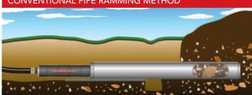
Pipe Ramming is an excellent, cost efficient method for placing steel casing under roads, railroads, finished landscapes and structures. The casing is installed open ended and cleaned out after installation is complete.
