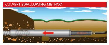
Replace deteriorating or over capacity culverts without disruption to roads, railroads, and other structures. Ram a steel casing over the existing culvert and clean out to complete the installation.
