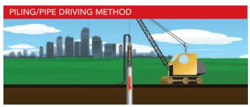
HammerHead rammers are a cost effective means to drive steel casings vertically, creating foundations or ground stabilization pilings.
