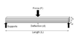
This test is used to measure the horizontal strength of the material. Supports are placed under the sample at each end, and then a piston drives down at the center. The force to drive down and the amount of deflection are measured to come up with the specimen's "Flexural Modulus".
